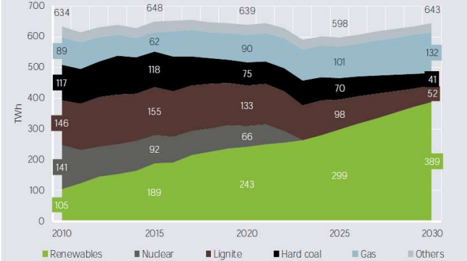
Figure S-3: Gross electricity generation in 2010-2030 with implementation of the coal compromise
