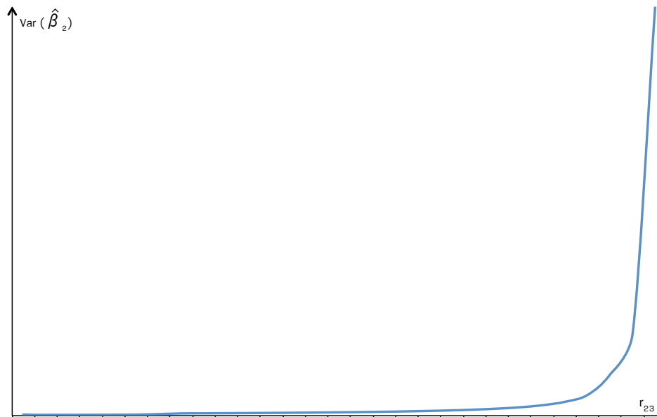
Figure 10.1: The consequence of an increase in the correlation coefficient on the variance estimators
